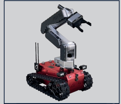
ARM (LIFT CAPACITY: 70KG / 154 LBS)
