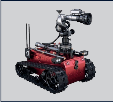
WATER / FOAM MONITOR
