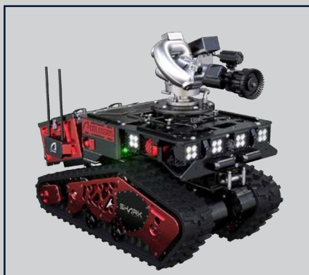
WATER / FOAM MONITOR
